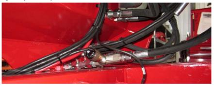
Less flow means the shut off responds quicker but lift will be fractionally slower. More open, will result in a quicker lift but will mean the shut off ram becomes lazy and could result in over-seeding at the end of each run and delays, therefore under-seeding at the start of each run.
