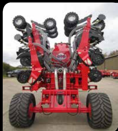
Unique lift and fold system of the wings and transport wheels on a simple heavy duty pivoting mid-section headstock
