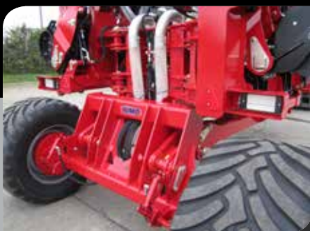
Heavy duty axles, 2.8m transport width
